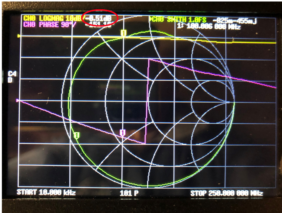
Figure 15-11: Reflection coefficient with open line @100MHz
