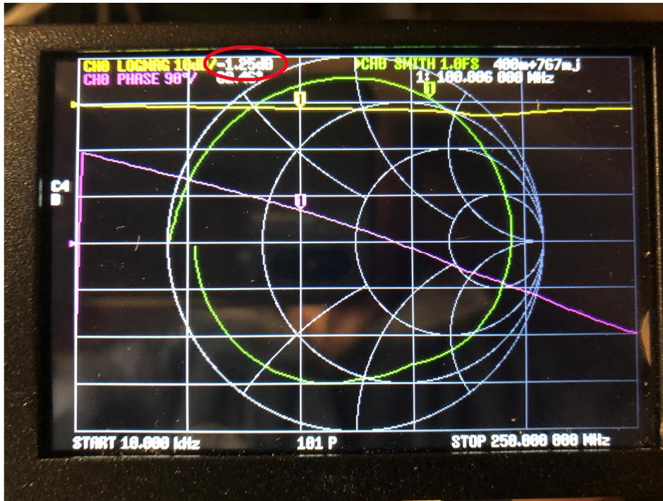
Figure 15-12: Reflection coefficient with shorted line @100MHz
