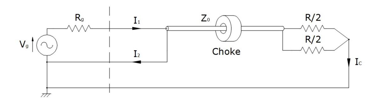
The blocking effect of a circuit made in this way is less pronounced than that of a resonant circuit, but it is not influenced by installation or external environmental factors. Moreover, the use of ferrite allows for the coverage of multiple frequency bands and sometimes even an entire frequency spectrum, such as in the case of HF.
