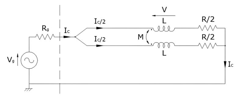
Usually, the common mode current,  $I_c$ , evenly splits between the two conductors of the line because the inductances L, produced by the choke, are equal and the load is balanced. Additionally, the coupling coefficient, k, of these inductances is very close to unity. As a result, the mutual inductance M $\approx$ L and the distributed inductance is very small. This is especially true when using coaxial cables, which is nearly always the case.
