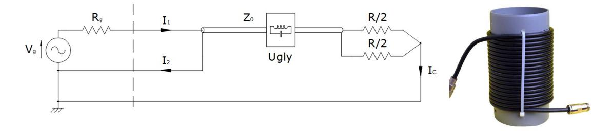
The blocking effect of such a circuit is very high at the resonance frequency because, typically, the circuit's Q is quite large. Unfortunately, its resonance frequency is influenced by installation and external environmental factors. Moreover, due to the high Q, these devices are not capable of effectively covering more than two or three frequency bands.
