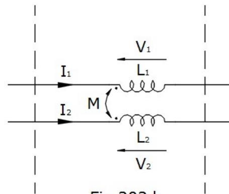
The choke is often built just by putting in a ferrite ring in the line, in a way that it coils both the two conductors (fig. 202a), but it can be obtained as well by coiling the line in air (we will get lower inductances). So, as a first approximation, the choke can be displayed with a couple of inductances  $L_1$  and  $L_2$  mutually paired one to the other  $M$ , figure 202b.
